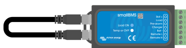
Testing a Small BMS by connecting a single BMS extension cable to both BMS cable connections
