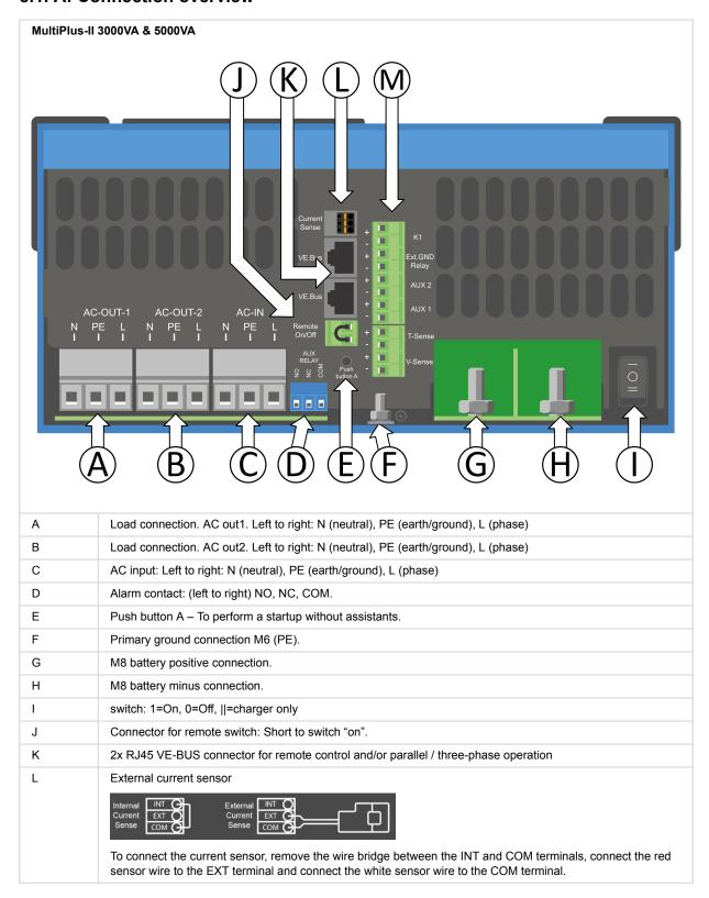
Μ Terminal for: top to bottom: 1. 12V 100mA 2. Programmable contact K1 open collector 70V 100mA External ground relay + 3. External ground relay -4. 5. Aux input 1 + Aux input 1 -6. 7. Aux input 2 + Aux input 2 -8. Temperature sense + 9. 10. Temperature sense -11. Battery voltage sense + 12. Battery voltage sense -
